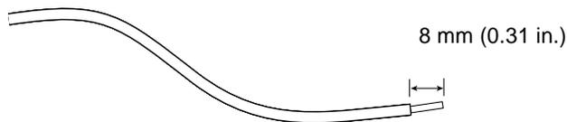
FIGURE 3-1 Stripping the Insulation From the Wire
